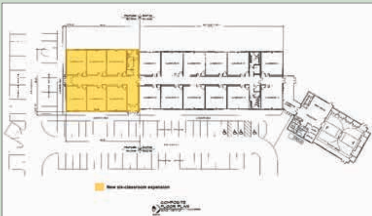
The expansion of Notre Dame's lower division will add six new classrooms, a restroom and a new entrance/exit to the south end of the existing classroom building.
